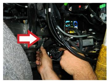
**STEP 2:** Reattach all air line fittings to the compressor assembly.
