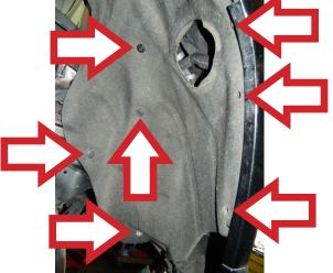
**STEP 7:** Remove other push type fasteners & bolts that secure fender liner (splash shield).
