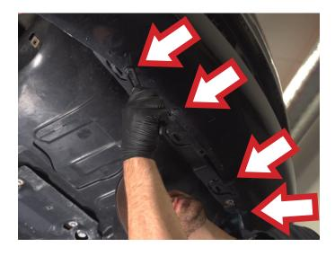
**STEP 10:** Disconnect the filter retaining clip from the body, and the hoses from the routing clips. Feed the filter retaining clip through the hoses as you're disconnecting the rerouting clips. Finally, disconnect the two compressor wiring harness connectors. **NOTE:** Pay particular attention to the routing of the hoses. There can be no twisting or kinking of the hoses when reassembled.
