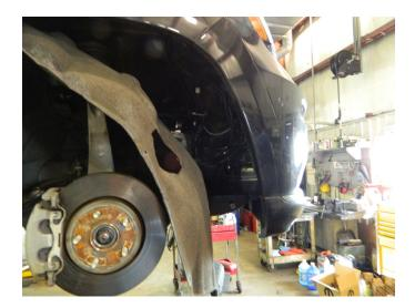
**STEP 8:** Remove the right front wheel splash shield.
