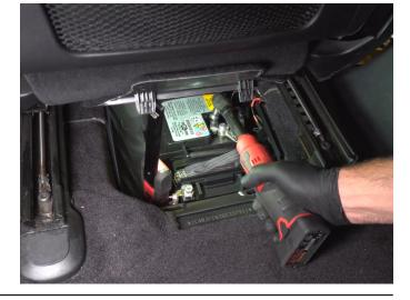
**STEP 12:** Using a nitrogen tank and suspension fill tool, refill the reservoir. Hook the suspension fill tool up to the fitting on the reservoir behind the rear driver's side seat. Set the tank regulator at 12 bar (175 psi).
