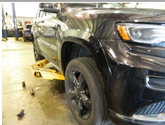
**STEP 3:** Using a diagnostic scan tool, do a complete system deflate to the atmosphere. **NOTE:** Some scan tools may use different terminology than what is indicated here.
