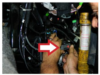
**STEP 11:** Using a 13mm wrench, disconnect the four air spring lines. **NOTE:** Mark the lines with their corresponding port before removal, to aid with install.
