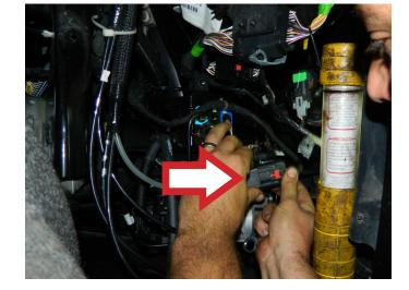
**STEP 5:** Connect the compressor wiring harness connector.
