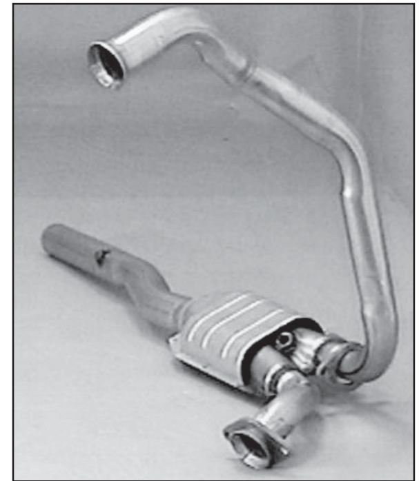
Catalytic Converter for a Dodge Ram
