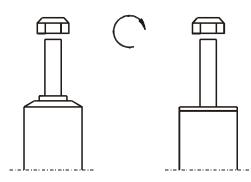
Do not use an impact tool to loosen or tighten fasteners due to possible damage to the product. Self- locking nuts must only be used once!
