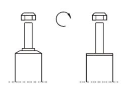
Do not use an impact tool to loosen or tighten fasteners due to possible damage to the product. Self-locking nuts must only be <u>used once!</u>
