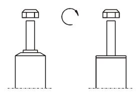
Do not use an impact tool to loosen or tighten fasteners due to possible damage to the product. Self-locking nuts must only be used once!
