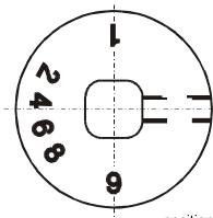
position **9 = comfort** ( clockwise direction) position **1 = sport** ( counter- clockwise direction)
