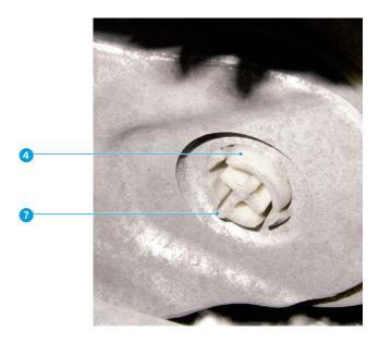
Rotate air spring approximately 30° anti-clockwise to loosen the upper connection and remove downwards
