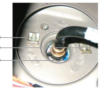
Unfasten retaining clip at wheel carrier and remove air spring ④.
