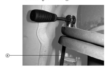
■ Dismantle level sensor linkage ④.
