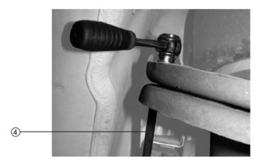
■ Dismantle level sensor linkage ④.
