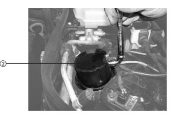
■ Screw off pressure line union on strut ②.
