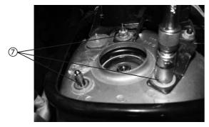
■ Push the bottom track control arm down and remove the strut sideways and downwards.
