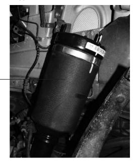
■ Assemble strut fork to the bottom track control arm ⑨.
