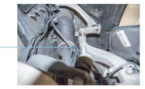
Disconnect the screw connection and dismantle the stabiliser's coupling rod 4 at the steering knuckle
