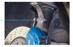
Disconnect the upper transverse link 5 from the steering knuckle 6 and secure the steering knuckle appropriately
