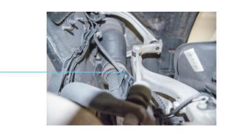
Disconnect the screw connection and dismantle the stabiliser's coupling rod 4 at the steering knuckle
