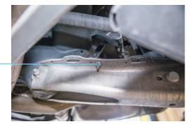
Disconnect the air suspension module's connecting wire 10 and decouple it from the bracket
