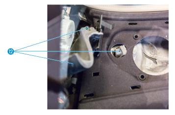
Pull the air suspension module downwards and remove
