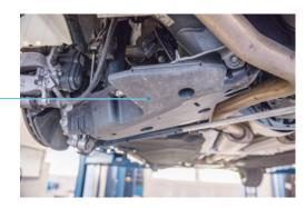
Disassemble the connection to the height sensor 9 at the traverse link
