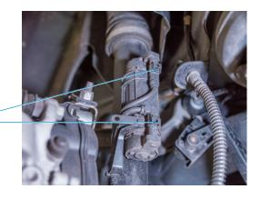
Disconnect the screw connection (1) on the transverse link and dismount the transverse link
