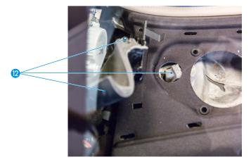
Pull the air suspension module downwards and remove
