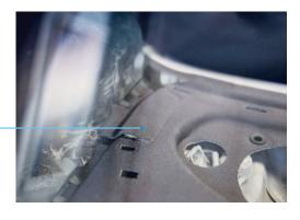
Using a suitable tool, carefully cut into the insulation underneath 6 at the edge of the parcel shelf along the markings shown and/ or carefully cut into the pre-existing perforations on the component and fold back, paying attention to the electrical wires
