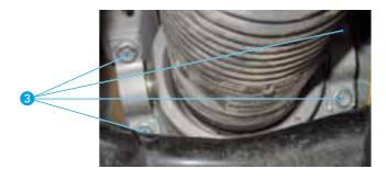
Loosen screw connection on spring strut 4
