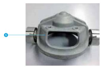
Insert cable adapter 6 in the parallel damping adjustment unit of the BILSTEIN spring strut and fasten to the welding stud on the shock absorber using the enclosed cable clip 7
