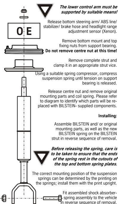
All rubber- mounted strut/ damper attachments must not be fully tightened until AFTER the suspension system is loaded (wheels on the ground). Other mounting fasteners (for example brackets) must be securely tightened BEFORE load is placed on the suspension system.
