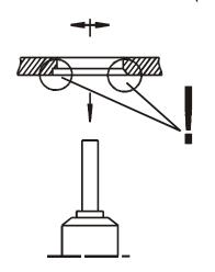
When fitting the spring plate (  $\bf 1$  ) care must be taken to ensure that the circlip ring (  $\bf 2$  ) is seated correctly!
