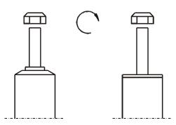
All rubber- mounted strut/ damper attachments must not be fully tightened until AFTER the suspension system is loaded (wheels on the ground). Other mounting fasteners (for example brackets) must be securely tightened BEFORE load is placed on the suspension system. Do not use an impact tool to loosen or tighten fasteners due to possible demage to the product.
