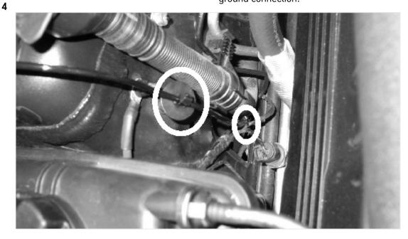
Replace the plastic cover of the strut on the dome. Attach the new plug housing of the adapter cable to the free slot on opposite side. The original plug housing remains in its original place.
