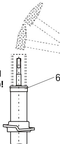
When fitting the spring plate ( 1 ) care must be taken to ensure that the circlip ring ( 2 ) is seated correctly!
