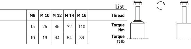
DO NOT USE IMPACT TOOLS FOR LOOSENING OR TIGHTENING FASTENERS, BECAUSE THIS MAY DESTROY THE THREADS. SELF- LOCKING NUTS MUST ONLY BE <u>USED ONCE</u>!
