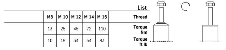
DO NOT USE IMPACT TOOLS FOR LOOSENING OR TIGHTENING FASTENERS, BECAUSE THIS MAY DESTROY THE THREADS. SELF- LOCKING NUTS MUST ONLY BE <u>USED ONCE</u>!
