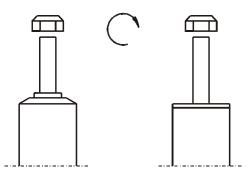
Do not use an impact tool to loosen or tighten fasteners due to possible damage to the product.
