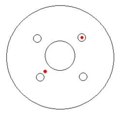
Measure runout and record results once again. If the results from both measurements match in both location and amount of runout measured, then excessive runout exists in the rotor itself, and the rotor requires either replacement or machining.
