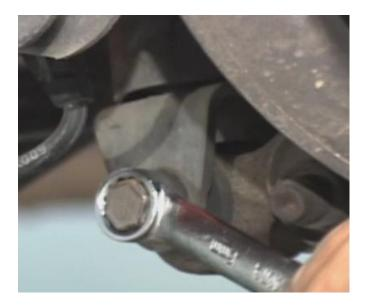
• Remove the top mounting hardware from the old shock.
