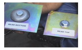
Install the supplied bottom spring support by putting the bolt and washer through the bottom of the spring seat. Install the plate and hardware on top of the spring seat.
