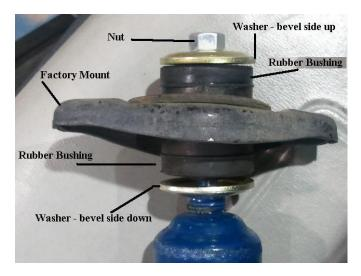
Install the rear shock bottom mount first.
