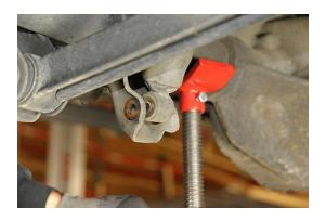
• Remove the air spring retaining clip.
