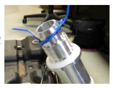
**STEP 8:** Place the new inlet valve into tank opening.
