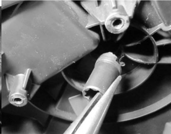
Figure 11- Removing Door Shaft
