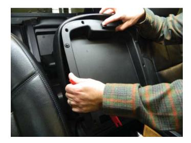
**STEP 4:** Press the latch through the hole to remove the underside of the console lid from the console.
