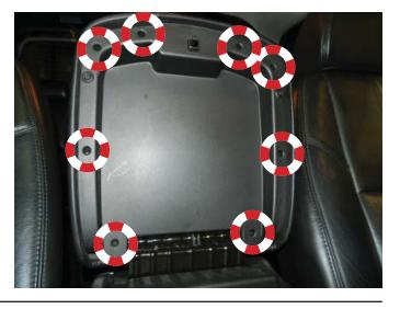
**STEP 4:** Verify that all of the hardware is secure and close the console lid to ensure that it latches properly.
