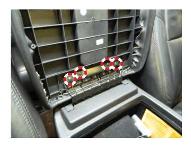
**STEP 2:** Press the underside of the console lid onto the console, making sure to feed the latch through the hole at the top.
