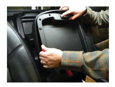
**STEP 5:** Using a Phillips screwdriver or power screwdriver with Phillips attachment, remove the four (4) screws to disconnect the top of the console lid from the center console.
