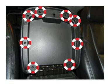
**STEP 3:** Using a plastic pry tool or flat-blade screwdriver, pry the underside of the console lid from the console.
