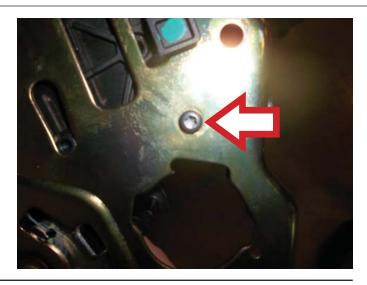
**STEP 4:** Using a 10mm socket and ratchet assembly, install the three (3) lift gate latch bracket retaining screws.
