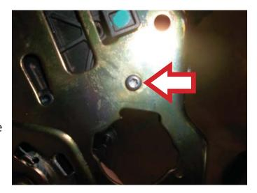
**STEP 6:** Slide the lift gate lock actuator toward the passenger side of the vehicle, to release the actuator from the lift gate latch retaining bracket. Once the actuator is disconnected from the bracket, slide the lift gate actuator arm out of position.
