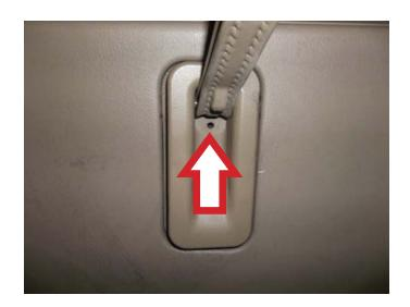
**STEP 8:** Verify that the lift gate lock actuator is operating properly and that the interior trim panel is secure.
