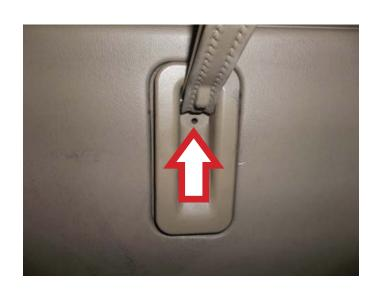
**STEP 2:** Using a trim panel removal tool, remove the upper portion of the interior lift gate panel assembly. Once the upper portion of the interior trim panel has been removed, disconnect the lower portion of the interior trim panel.
