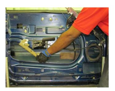
**STEP 10:** Remove the three (3) window lift motor attaching screws.
