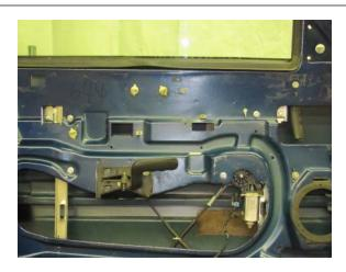
**STEP 8:** Tighten the six 10mm regulator mounting bolts in the following order: Bolt A, D, C, F, B, E. Tighten the bolts to 9 N-m (80 lb in).
