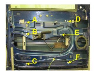
STEP 9: Lubricate the window run channels.
