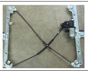
**STEP 2:** Install the left side track into the door.
