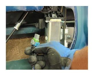
**STEP 6:** Remove tape or wedge from the window and door frame and lower window into the window guide clamps making sure that the window is correctly seated in the guides.
