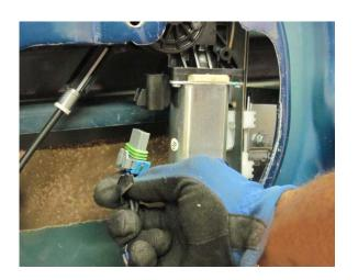
**STEP 7:** Remove the six 10mm window regulator mounting bolts that secure the window regulator to the door frame.
