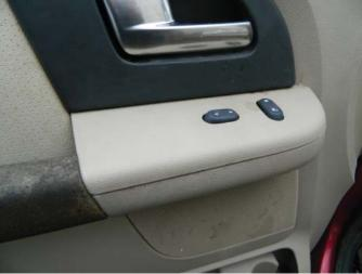
**STEP 15:** Install the power switch assembly.
