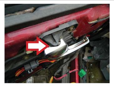
**STEP 10:** Temporarily connect the window switch to lower the door glass, exposing the two (2) bolts mounting the door glass to the window regulator. You will be using a 10mm socket with extension and a ratchet.
