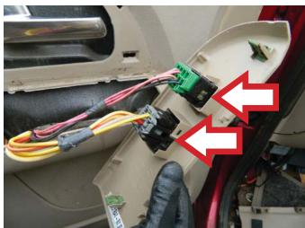
**STEP 4:** Disconnect the switch panel assembly.
