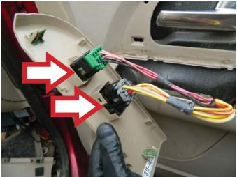
**STEP 4:** Disconnect the switch panel assembly.
