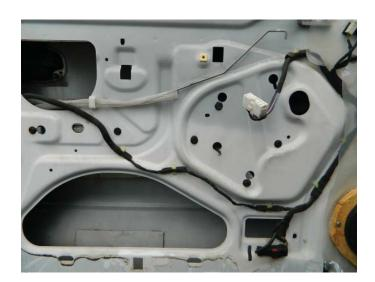
**STEP 6a:** Temporarily connect the master power switch assembly and lower the window glass to expose the window regulator mounting screws. Remove the mounting screws.
