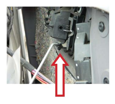
**STEP 4:** Disconnect the master power switch assembly.
