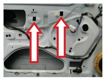
**STEP 4a:** Attach the window glass to the window regulator.
