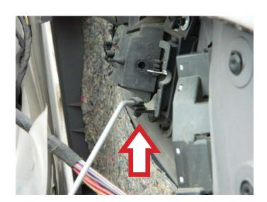
**STEP 8:** Connect the master power window switch assembly.
