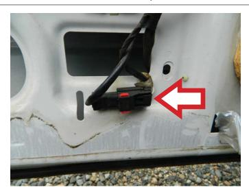
**STEP 4:** Temporarily install the master power window switch so that you can lower the door glass to meet the attaching mounts on the window regulator.
