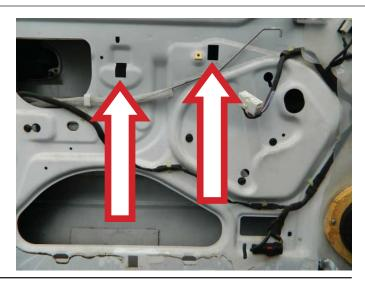
**STEP 7:** Disconnect the window lift motor connector.
