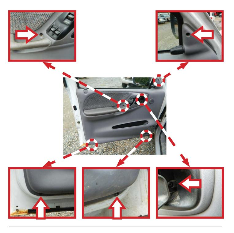
**STEP 11:** Verify that all of the interior door trim panel retaining screws are tight and that the window regulator is operating properly.
