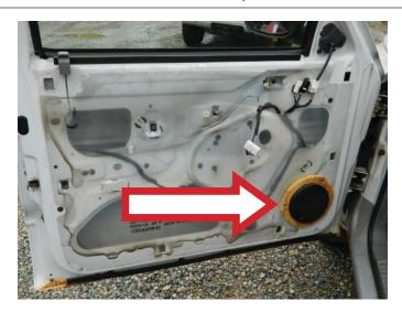
**STEP 6:** Remove the water vapor barrier.
