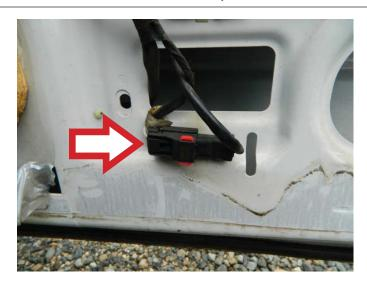
**STEP 4:** Temporarily install the power window switch so that you can lower the door glass to meet the attaching mounts on the window regulator.
