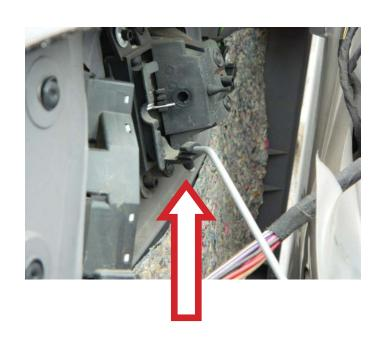
**STEP 8:** Connect the master power window switch assembly.
