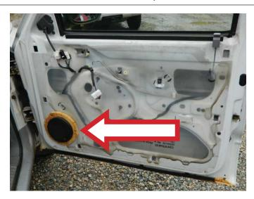
**STEP 6:** Remove the water vapor barrier.
