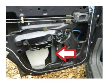
**STEP 2:** Connect the window lift motor connector.
