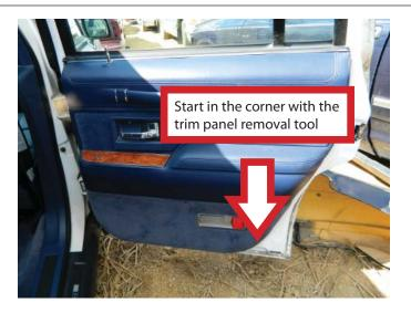
**STEP 6:** Remove the interior door trim panel from the door. **NOTE:** USE CAUTION WHEN REMOVING THE INTERIOR DOOR TRIM PANEL. THE COURTESY LAMP WILL STILL BE ATTACHED.
