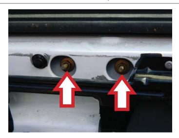
**STEP 13:** Disconnect the window lift motor and remove the window regulator assembly through the main access opening in the door.
