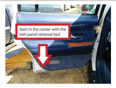
**STEP 6:** Remove the interior door trim panel from the door. **NOTE:** USE CAUTION WHEN REMOVING THE INTERIOR DOOR TRIM PANEL. THE COURTESY LAMP WILL STILL BE ATTACHED.
