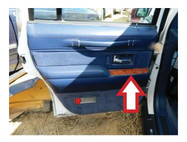
**STEP 9:** Attach the power switch assembly onto the interior door trim panel.
