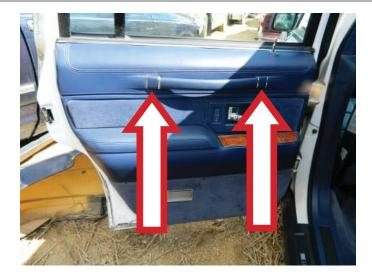
**STEP 12:** Verify that the window regulator assembly is operating properly and that all of the interior door trim panel retaining screws are tight.
