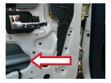
**STEP 14:** Remove the three (3) window lift motor attaching screws and remove the window lift motor from the window regulator.
