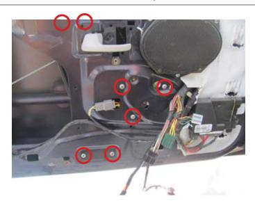
**STEP 13:** Remove the bolts that attach the window glass to the regulator.
