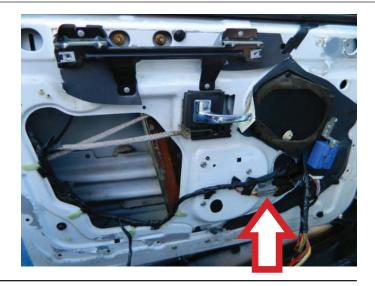
**STEP 4:** Manually slide the door glass to align the door glass mounts with the attaching points on the window regulator. **NOTE:** Dorman hardware kit 702-013 has the proper bolts to use in place of the original rivets that attached the door glass to the window regulator.
