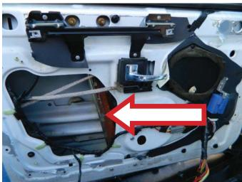
STEP 14: Remove the three (3) window lift motor attaching bolts.
