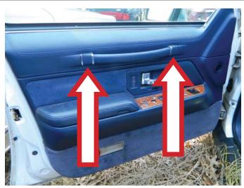
**STEP 3:** Using a Phillips head screwdriver, remove the interior door pull retaining screws.
