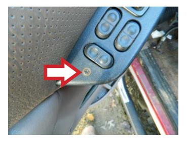
**STEP 11:** Attach the master power window switch to the interior door trim panel.
