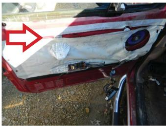
**STEP 5:** Attach the water vapor barrier.
