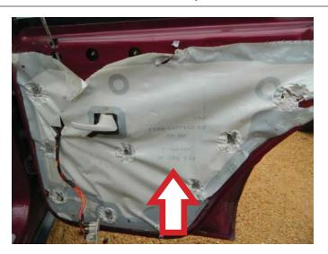
**STEP 6:** Place the power window switch through the opening on the interior door trim panel.
