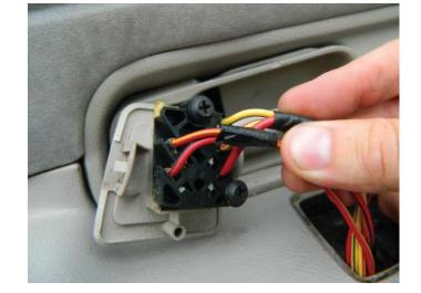
**STEP 6:** Place the power window switch through the opening on the interior door trim panel.
