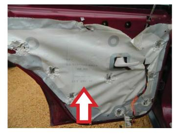
**STEP 5:** Attach the water vapor barrier.
