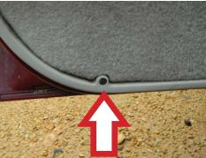
**STEP 2:** Using a trim panel removal tool, remove the door handle bezel.
