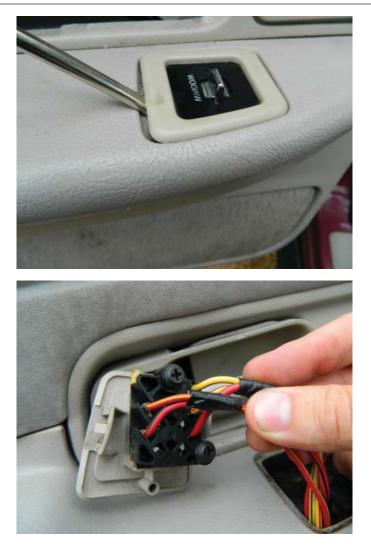
**STEP 4:** Lift the interior door trim panel in an upward and outward motion to remove the door trim panel. **NOTE:** Before lifting the door trim panel from its position, you may want to push the window switch through the opening of the door trim panel.
