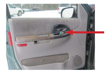
**STEP 15:** Install the power master door switch assembly.
