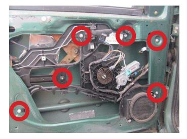
**STEP 10:** Remove the window regulator module assembly.
