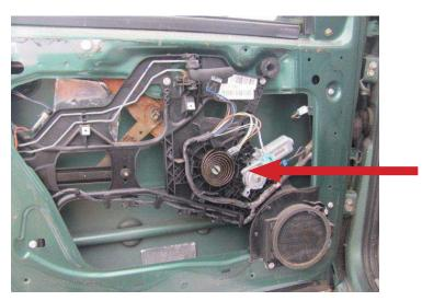
**STEP 6:** Disconnect the electrical connector at the window lift motor.
