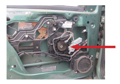
**STEP 5:** Attach the window regulator door assembly onto the door.
