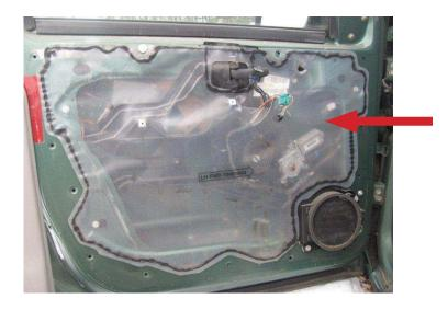
STEP 12: Install the water barrier shield.
