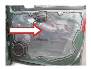
**STEP 13:** Align the door trim panel retainers. With light to moderate pressure, push the door panel into position.
