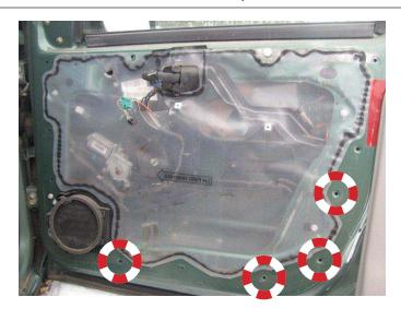
**STEP 3a:** Using either the saddle cup assembly, tape, or wedge, attach to the door glass to prevent the glass from falling.
