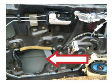
**STEP 2:** Slide the window lift motor connector through the access hole.
