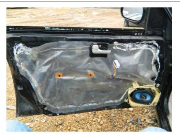
**STEP 7:** Install the water vapor barrier.
