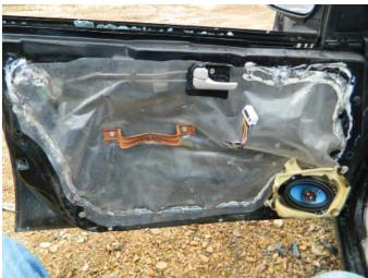
**STEP 8:** Remove the water vapor barrier.
