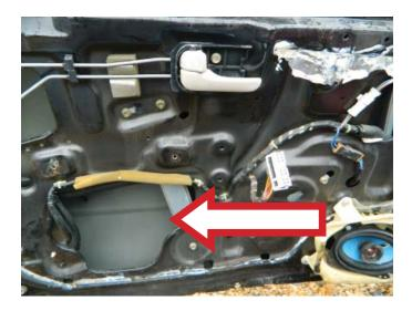
**STEP 15:** Remove the window regulator assembly through the main access hole.
