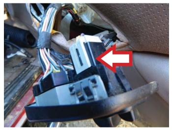
**STEP 3:** Once the interior door trim panel has been removed from the door, remove the master power switch assembly by lifting from the door trim panel and placing the master power switch assembly through the hole in the interior door trim panel.
