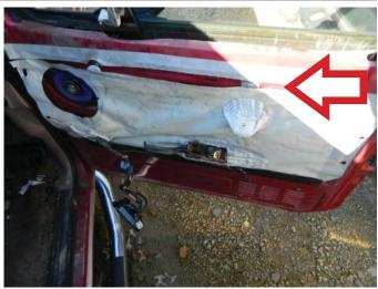
**STEP 5:** Attach the water vapor barrier.
