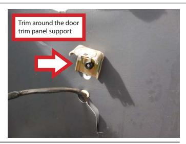
**STEP 7:** Using a razor knife or razor blade, trim around the door speaker. **NOTE:** THIS DOES NOT APPLY TO ALL VEHICLES. MOST WATER VAPOR BARRIERS WERE PRE-CUT FOR THE SPEAKER OPENING.
