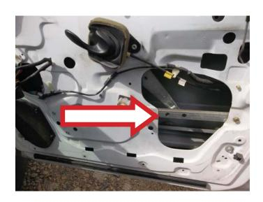
**STEP 2:** Using a 10 mm socket and ratchet, attach the window regulator rail to the door.
