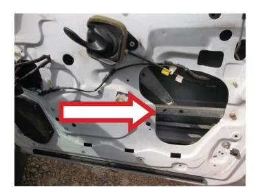
**STEP 15:** Remove the three (3) window lift motor attaching bolts. **NOTE:** SOME VEHICLES CAME EQUIPPED WITH RIVETS ATTACHING TO THE WINDOW REGULATOR. IF THIS IS THE CASE, FOLLOW THE WINDOW REGULATOR RIVET REMOVAL SECTION OF THE INSTRUCTIONS. **CAUTION:** THE WINDOW REGULATOR ASSEMBLY IS UNDER EXTREME PRESSURE DUE TO THE WINDOW REGULATOR PRE-TENSIONER SPRING. REMOVE THE PRE-TENSIONER SPRING.
