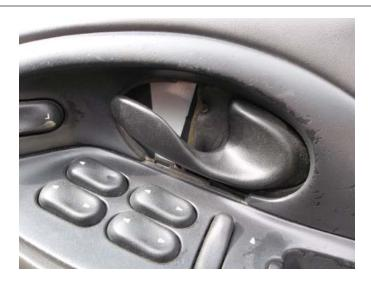
**STEP 3:** Using a trim panel removal tool, detach the interior door trim panel from the door. **NOTE:** THERE ARE INTERIOR DOOR TRIM PANEL RETAINERS EVERY TEN TO TWELVE INCHES. PLACE THE INTERIOR TRIM REMOVAL TOOL BETWEEN THE INTERIOR DOOR TRIM PANEL AND THE DOOR AND PULL THE REMOVAL TOOL TOWARD YOU TO RELEASE THE RETAINERS.
