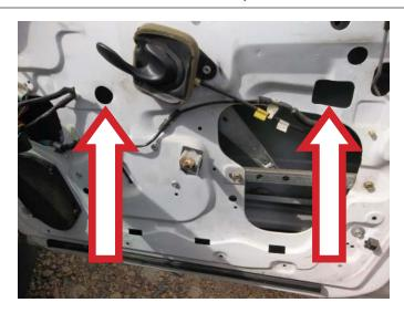
**STEP 10:** Using your 3/8" power drill and drill bits, remove the rivets attaching the door glass to the window regulator. **CAUTION:** USE EXTREME CARE WHILE DRILLING OUT THE DOOR GLASS ATTACHING RIVETS. FAILURE TO DO SO WILL RESULTS IN GLASS BREAKAGE. WHILE DRILLING THE RIVETS OUT, START WITH AN 1/8" DRILL BIT, WORKING YOUR WAY UP TO A 1/4" DRILL BIT. YOU ARE ONLY DRILLING THE HEAD OF THE RIVET. DO NOT DRILL ALL OF THE WAY THROUGH THE RIVET.
